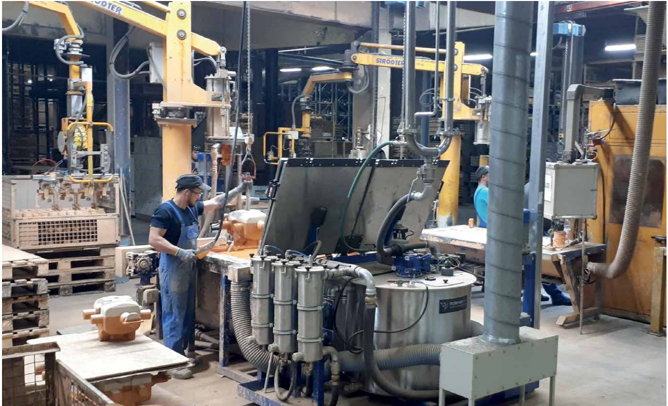
Coating a core at SLR in one of the new modernized coating dip tanks.
